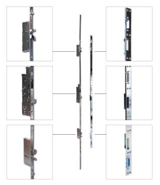
Featuring a centre hook and two steel anti-lift bolts, the Fullex XL uPVC door lock can be specified with two or four roller cams. The lock is extendable top and bottom as standard, making it highly versatile.
